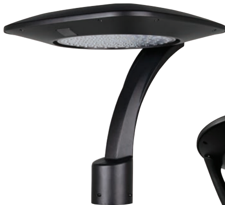
AeroLUX Single Arm Open Post Top Model# ALXR31 (Round) & ALXS31 (Square) Wattages: 41w & 72w Replaces up to 250w Optic: IES Types II, III, IV & V Delivered Lumens: 4,700-9,100
