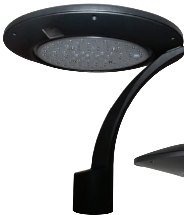
AeroLUX Single Arm Open Post Top Model# ALXR31 (Round) & ALXS31 (Square) Wattages: 41w & 72w Replaces up to 250w Optic: IES Types II, III, IV & V Delivered Lumens: 4,700-9,100
